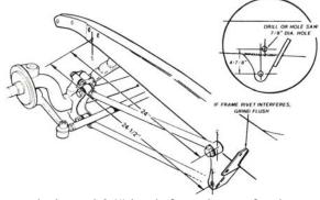
frame bracket. Upper hole is located 4 7/8" above lower hole and 24" back from lower fender brace hole on frame.
